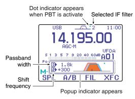
•[PBT] controls should normally be set to the center positions (PBT setting is cleared) when there is no interference.
